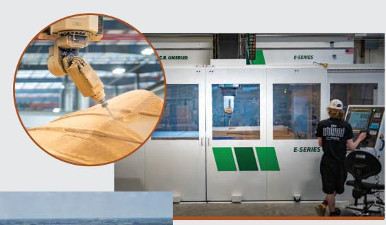
The MBI TOOLING DEVEOLPMENT CENTER is a new state-of-the-art facility that provides safe, predictable and meticulously engineered tooling for use across our brands. For example, our custom 5-axis router enables precise construction of key molds. Technologies like this enable better quality and also faster time to market for new products.
