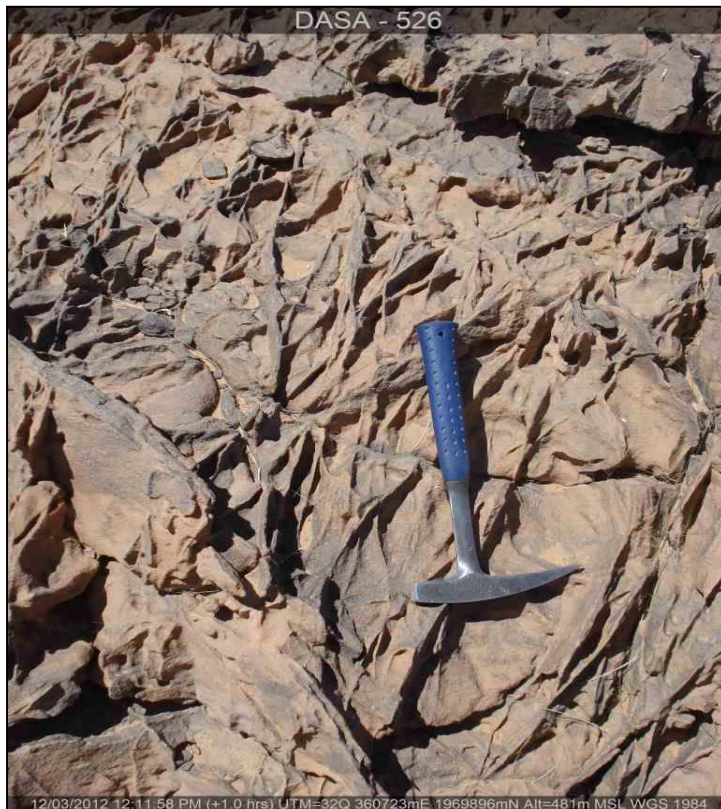
Figure 7-15: Heavily quartz veined Tegama sandstone; mount inside the Assouza Graben Source: GAFC
