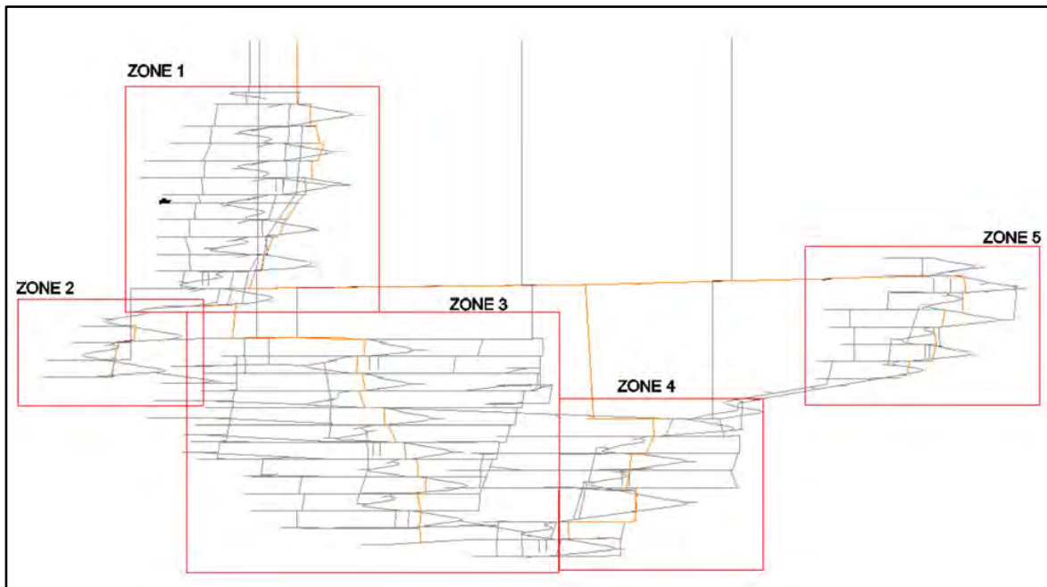
Figure 18-17: Schematic Showing Underground Backfill Piping Distribution.
