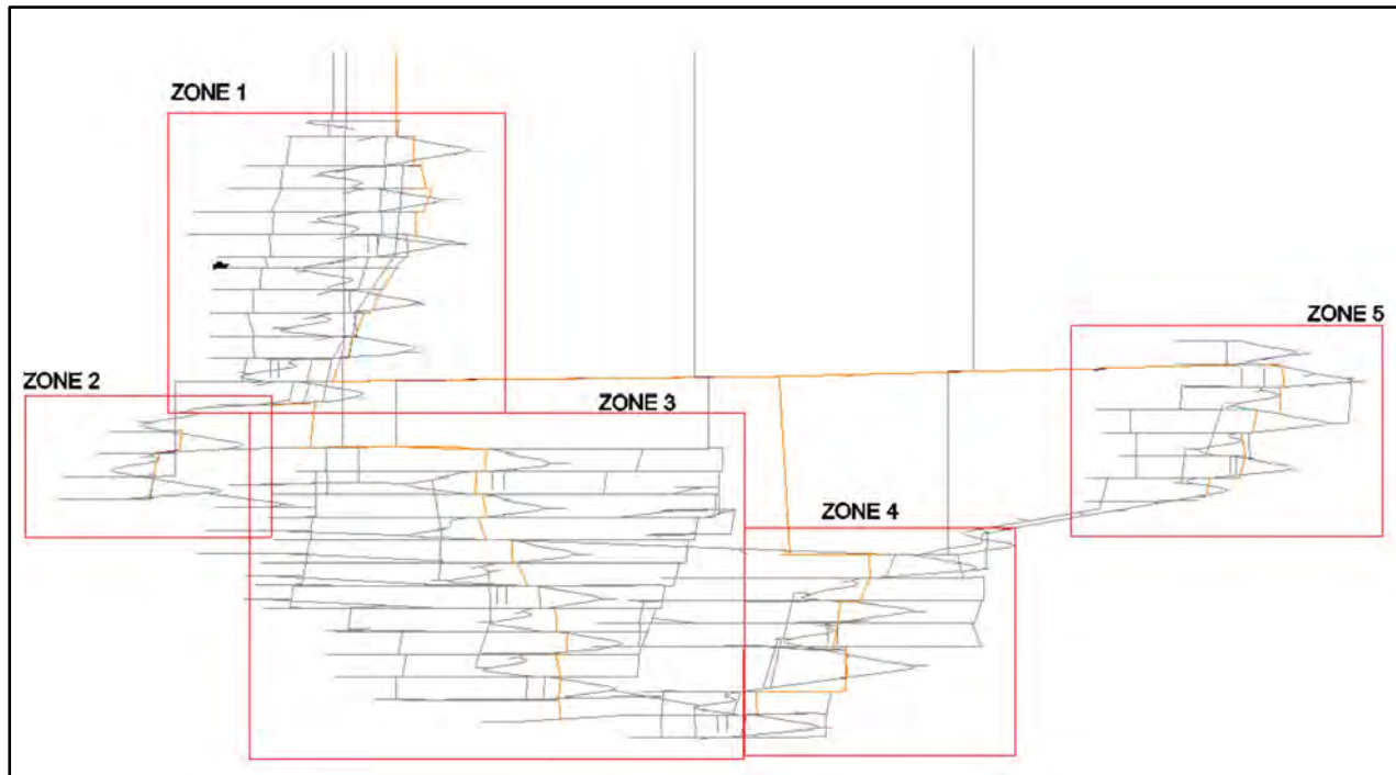
Figure 18-18: Schematic Showing Underground Backfill Piping Distribution.
