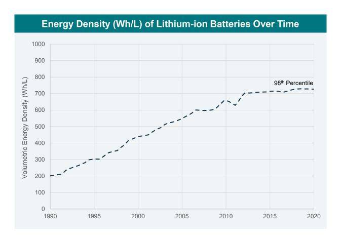
This chart shows the increases in energy density of the top-performing commercial lithium-ion batteries over time; the trend line represents the 98th percentile (top 2%) of battery performance in volumetric energy density. Source: Energy Environ. Sci., 2021,14, 1635-1651.
