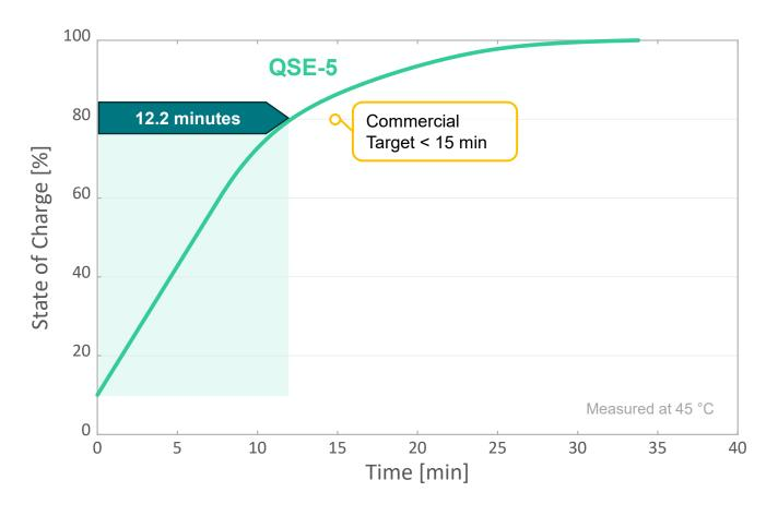
C/3 (1.87 mA/cm²) charge rate from 0-10% SOC, 4C (22.4 mA/cm²) charge rate from 10% to upper cut-off voltage (4.25V). Commercially relevant dimensions may vary from 60x75 mm to 70x85 mm, depending on cell format.
