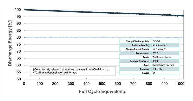
Note: Test data sourced from the Volkswagen Group's PowerCo testing lab in Germany from the top-performing A0 prototype cell. Full cycle equivalent is defined by PowerCo as the overall discharge capacity throughput divided by the nominal discharge capacity.
